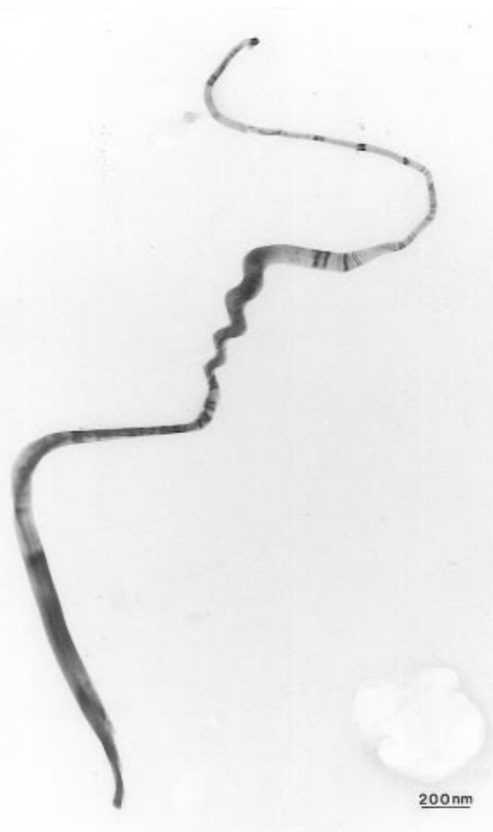
Figure 7. TEM image of a single twisted filament of crystalline \text{BaSO}_4 formed in supersaturated microemulsions ( w = 66 , [\text{AOT}] = 0.27 \text{ M} ) produced by rapidly mixing preformed \text{AOT}/\text{isooctane}/\text{H}_2\text{O} microemulsions containing 0.01 M \text{Ba}^{2+} or 0.01 M \text{SO}_4^{2-} at room temperature.
